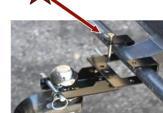
When hauling trash cans we suggest height between 14"- 21" allowing for approximately 30% of the cans weight to be resting on the support
